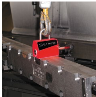
Model 300: Cast part on machining centre
