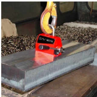
Model 150: Milling machine loading and unloading
